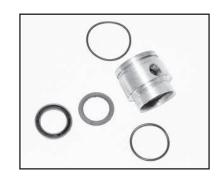
**11.** Inspect o-rings (#21 and 22) and replace as necessary.
