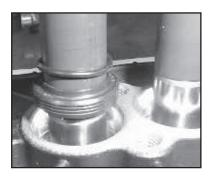
14. If the oil seals (#19) were removed, replace them with the primary seal lip (grooved side) towards the crankcase and the dust lip (tapered end) towards the valve casing (#26). Lubricate the seal before replacing. Install the oil scraper (#18) over the plunger.
