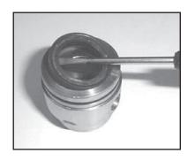
**10.** Remove the weep grooved seals (23A) from the seal case (#20). Remove the pressure rings (#24).
