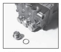
1. With a 24mm socket wrench, remove the (3) discharge valve plugs and (3) inlet valve plugs (#32). Inspect the o-ring (#33) for wear and replace if damaged.
